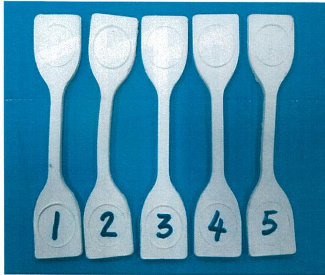
Figure 1. Photograph of sample 'VT-620 LM MS Sealant' – Before test
