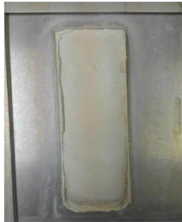
MS sealant QUV test result
