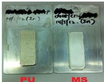
ASTM C 1442-06 (QUV test)
