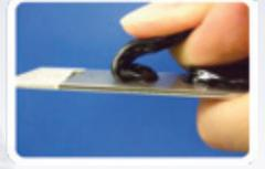
Adhesive Failure (Silicone Sealant)
