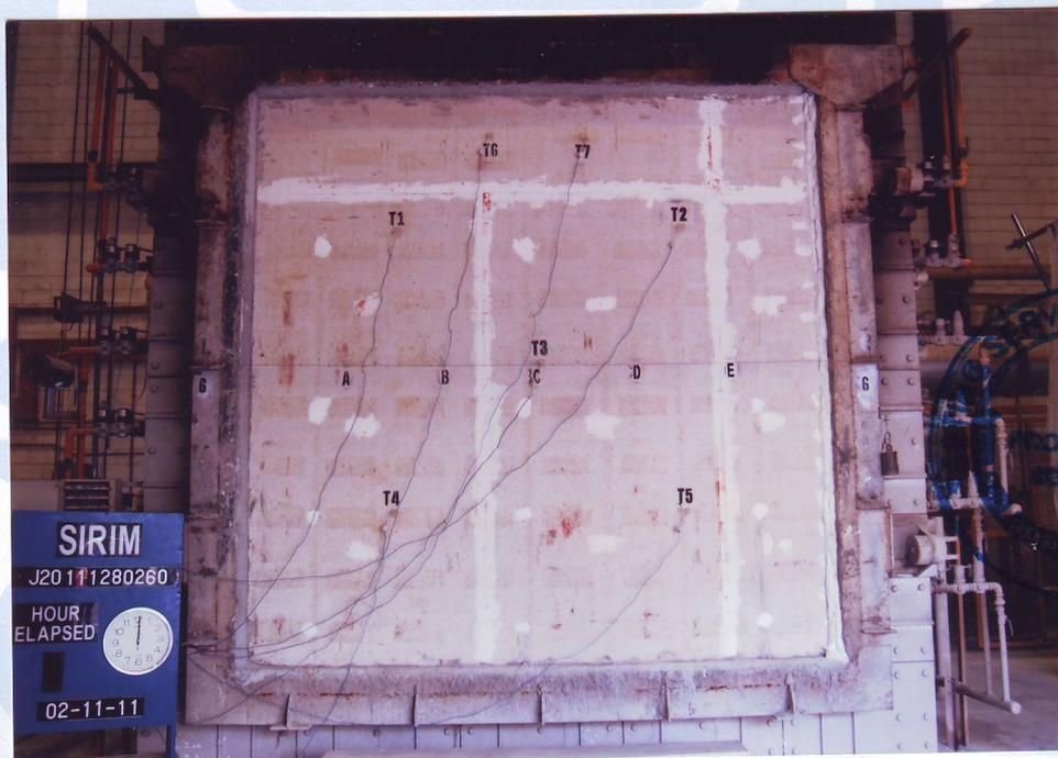
Photo 2: The unexposed face of the partition system before the test
