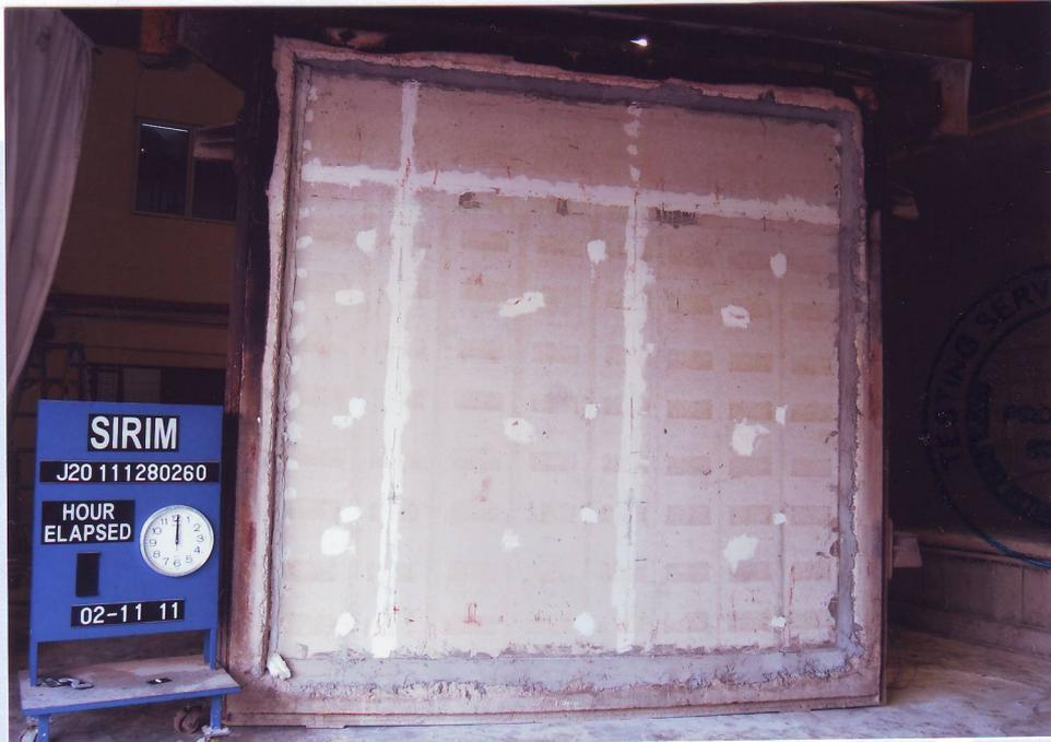
Photo 1: The exposed face of the partition system before the test
