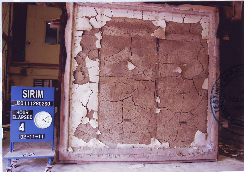
Photo 12: The exposed face of the partition system after the test
