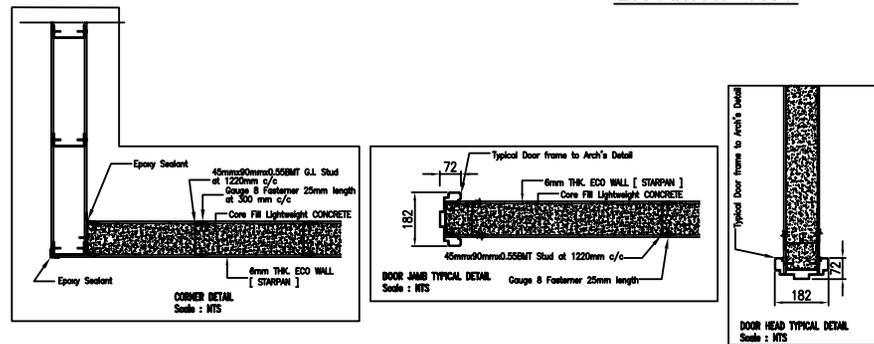
**DETAIL FOR INTERNAL ECO WALL 102MM THICK**
