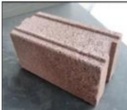
Figure 1.0: Full Interlocking Brick
